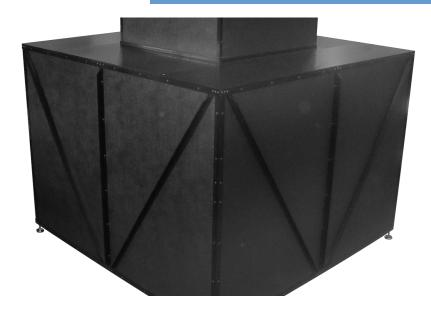
Sciencetech's flash solar simulators are designed to test large photovoltaic devices up to  $2m \times 2m$  (79"  $\times$  79") in size. It uses a heavy duty xenon flash lamp and AMI.5G calibrated solar filter to approximate the sun's true spectral distribution following ASTM E927-10 Class A standards. The simulator fires short flashes of light to avoid heating a photovoltaic device for measuring its performance.
