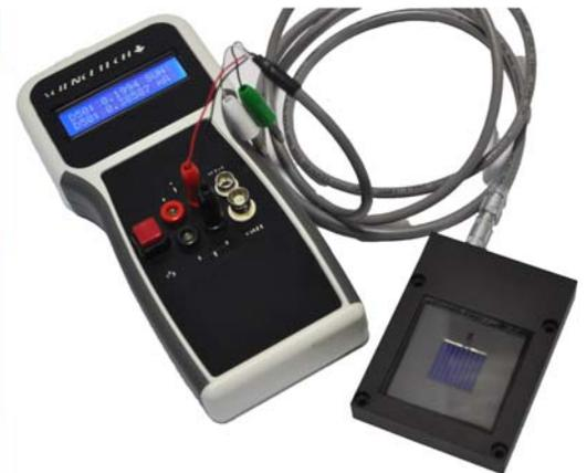
SOL-METER Digital Power Meter With SC-LT-Q NIST-Certified Reference Cell
