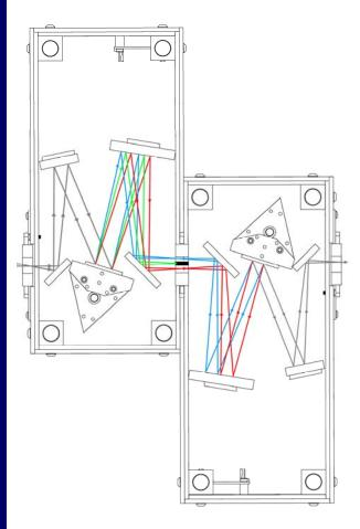
The 9072DS is made of 2 single monochromators in a **subtractive** mode: the dispersion of the second monochromator is in the opposite direction of that of the first one. The two gratings are mechanically connected and accurately motorized together. This leads to a spectrally homogenized beam at the output port of the second monochromator and greatly reduced stray light, ideal for spectroradiometry, Raman or UV measurements of solar radiation.
