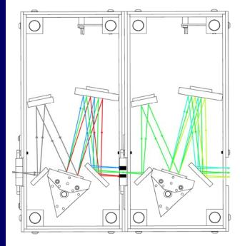
The 9072DA is made of 2 single monochromators in a **additive** mode: the dispersion of the second monochromator adds to that of the first one.
